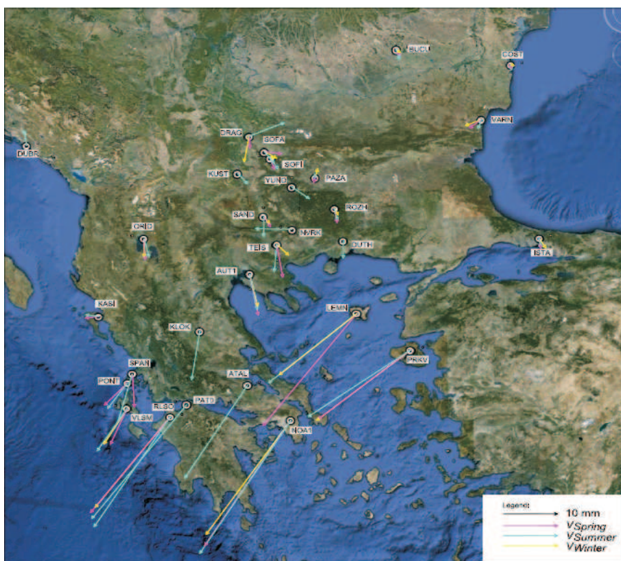
Fig. 3. Horizontal velocity vectors of BP stations for the three seasons with respect to the stable Eurasia
