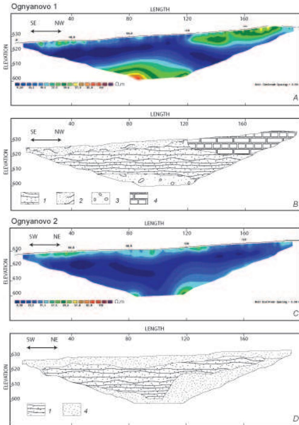
Fig. 2. Section, showing inversion results of resistivity data (A, C) and geological interpretation (B, D) of profiles near Ognyanovo. (Key: 1 – sandy clay; 2 – clayey sand and siltstone; 3 – coarse sand and gravel; 4 – diatomite)
