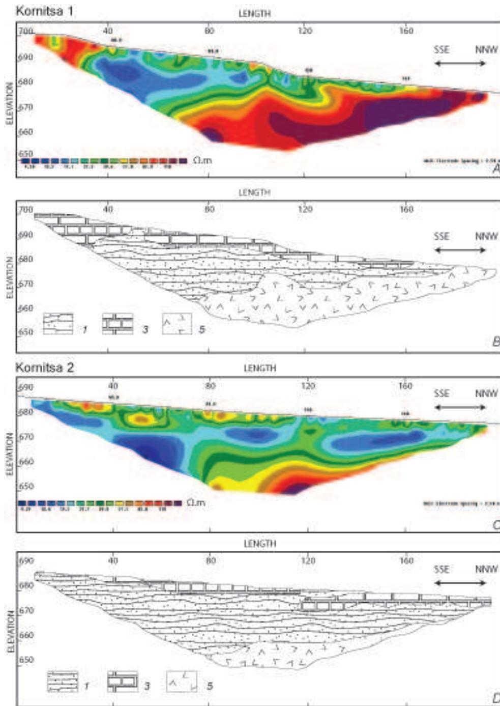
Fig. 3. Section, showing inversion results of resistivity data (A, C) and geological interpretation (B, D) of profiles near Kornitsa. (Key: 1 – sand and clay alternation; 3 – diatomite; 5 – volcanic rocks)
