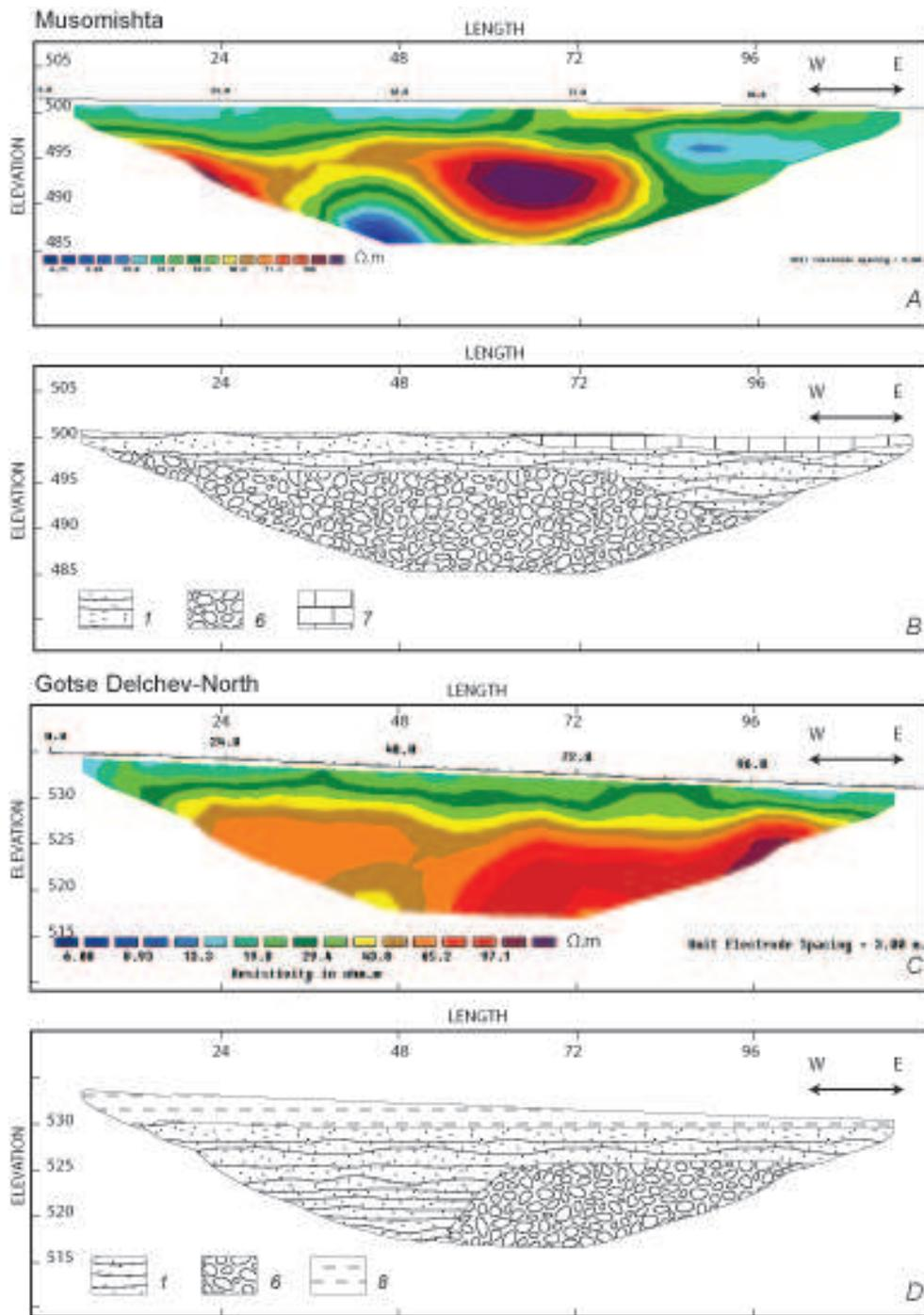
Fig. 4. Section, showing inversion results of resistivity data (A, C) and geological interpretation (B, D) of profiles Musomishta and Gotse Delchev-North. (Key: 1 – sand and clay alternation; 6 – conglomerate; 7 – travertine; 8 – clay)
