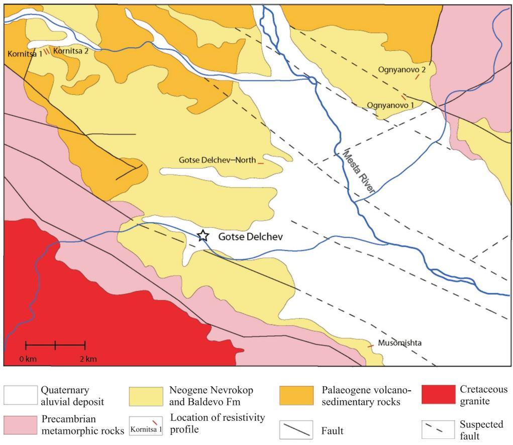
Fig. 1. Geological map (according to [10]) and location of the 2D resistivity survey lines
