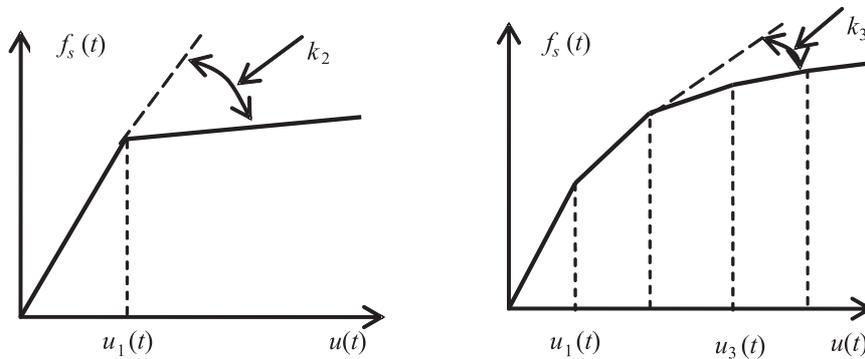
Fig. 1. Bi-linear or multi-linear  $f_s(x) - u(x)$  representation
