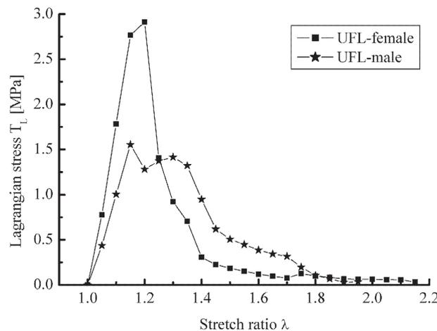
Fig. 1. Lagrangian stress-strain relationships between male and female samples cut in longitudinal direction L (number of female samples – 12, number of male samples – 9)
