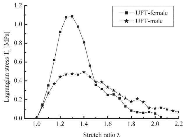
Fig. 2. Lagrangian stress-strain relationships between male and female samples cut in transversal direction T (number of female samples – 12, number of male samples – 9)
