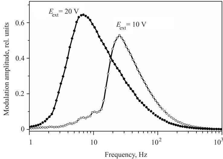
Fig. 3. The amplitude-frequency EO response (by light transmittance,  $\lambda = 632.8$  nm) of PDLC cell ( $10 \mu\text{m}$  thick). Spectra measured for two values of the applied voltage, under identical other experimental conditions. The temperature was kept at  $35^\circ\text{C}$
