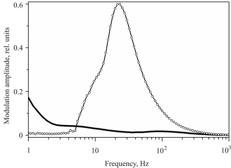
Fig. 2. EO modulation of laser light (wavelength  $\lambda = 632.8$  nm) transmitted through single-layered PDLC cells with a thickness of 10  $\mu\text{m}$ : with orthogonally rubbed teflon nanolayers on the ITO glasses (line with open circles); and without alignment layers on the ITO glasses (bold line). In both cases, the temperature of the PDLC cell was 35  $^{\circ}\text{C}$
