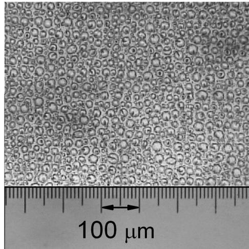
Fig. 1. Optical microscopy image (magnification  $\times 10$ ) of PDLC single layer with a thickness of  $10\ \mu\text{m}$  is studied here. The average size of the droplets is  $19.5\ \mu\text{m}$  (with a standard deviation of  $2.8\ \mu\text{m}$ )
